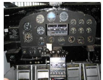
Original VFR Panel of Ford Tri-Motor 5-AT-74, N414H. Radio and transponder are modern but straight forward and simple.
